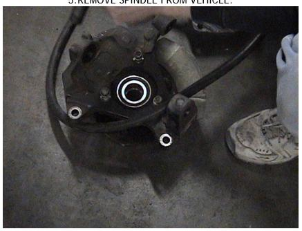
5. INSTALL M12 STUD SUPPLIED WITH SPINDLE INTO THE TOP THREADED MOUNTING HOLE OF SPINDLE. THIS STUD IS TO BE INSTALLED WITH LOCK-TIGHT AND TIGHTENED SECURELY.
