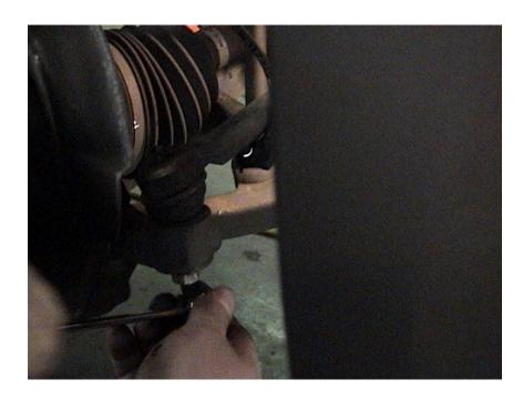
3-A. REMOVE CV AXLE. ( MARK CV BEFORE REMOVING )
