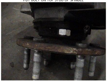
7. -A APPENDED CUT OFF THE EXCESS TOP BALL JOINT STUD FLUSH WITH THE NEW NUT ( I CUT 2 THREADS AFTER THE DISCOLORATION)
