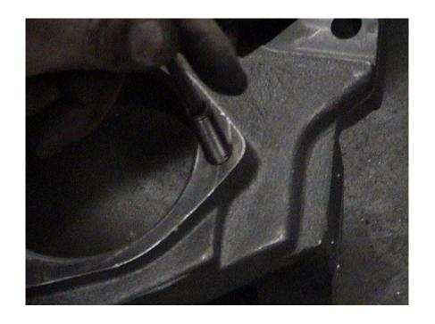
6. INSTALL HUB ASSEMBLY USING THE M12 STUD ON SPINDLE. (TIGHTEN TO 75 LBS) USE TWO OF YOUR ORIGINAL HUB BOLTS ON LOWER TWO HOLES, LOCK-TIGHT AND TIGHTEN THESE TWO BOLTS SECURELY (TIGHTEN TO MANUFACTURE SPECIFICATIONS.)
