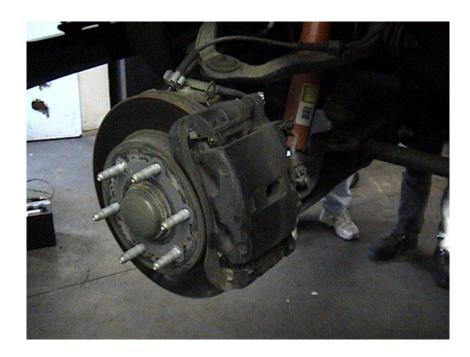
2. REMOVE HUB ASSEMBLY FROM SPINDLE.
